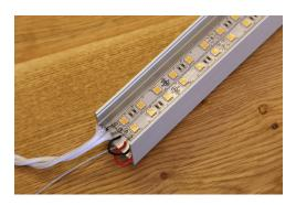
Connect the power wire to the tape, either by soldering or using a Tape Light Splice Connector.
