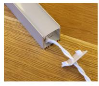
Put the cover in place by squeezing the sides and pressing the cover down into the grooves at the top of the channel, starting at one end and moving to the other.
